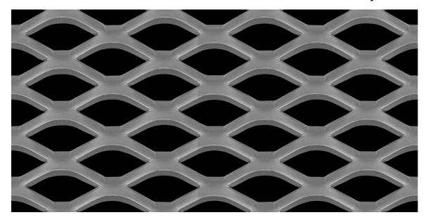
LW Pitch:38.10mmStrand Width:5.80mmSW Pitch:20.00mmThickness:4.00mmWeight:18.21 kg / m2Open Area:42%
